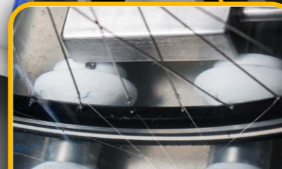
Ultrasonic cleaning for front and rear wheel with 4 immersion transducers
