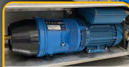
integr. High-performance blade compressor for operating of the Clean & Dry Gun
